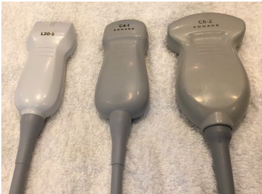
Figure 3.39 Linear probe and two curved array probes
