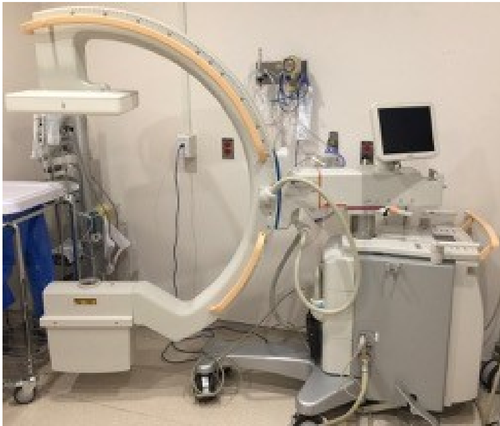
Figure 3.6D A Portable, Mini, C-Arm x-ray unit
