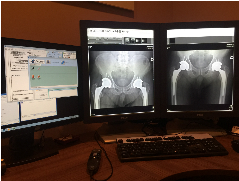
Figure 3.1 PACS Imaging Viewing Station (Workstation)
