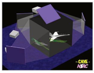
A diagram of the CAVE at the National Supercomputing Research Center (NSRC). The CAVE (CAVE Automatic Virtual Environment) was developed by DeFanti, et al at the University of Illinois. This CAVE installation is an enclosed 10 feet cube room-sized advanced visualization tool that combines high-resolution, stereoscopic projection and 3D computer graphics to create the illusion of complete immersion in a virtual environment.
