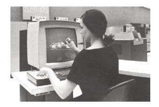
IBM developed three graphics related devices for DAC-1 — the 2250 display device, the 2280 film recorder, and the 2281 film scanner. The last two were discontinued because they were not received well in the industry.
