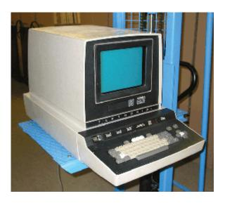
Tektronix 4002A Direct View Storage Tube Display
