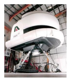
The physical simulator had a mock-up of the cockpit mounted on computer controllable pneumatic devices to simulate motion. The visual component of the simulator generated images that were presented to the training pilot on display devices mounted inside the physical simulator
