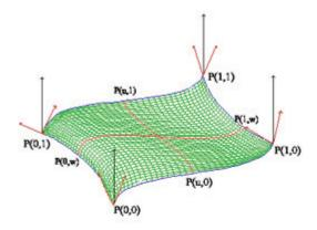
Graphic representation of the Coons' patch. The curvature on the interior is controlled by the geometry at the edges and the corners, with the depicted vectors providing the controls.
