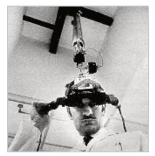
The ultrasonic head position sensor
