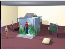
A diagram of the CAVE at the National Supercomputing Research Center (NSRC). The CAVE (CAVE Automatic Virtual Environment) was developed by DeFanti, et al at the University of Illinois. This CAVE installation is an enclosed 10 feet cube room-sized advanced visualization tool that combines high-resolution, stereoscopic projection and 3D computer graphics to create the illusion of complete immersion in a virtual environment.
