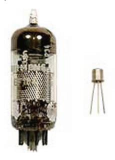
Vacuum tube and transistor
