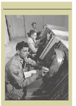
SAGE demonstrated pioneering solutions to the problem of the user interface. The system displayed extremely large amounts of information to its operators using the then-new cathode ray tube; operators could then obtain additional information on aircraft tracks by selecting them with a light gun. Similar techniques are still in use today.
