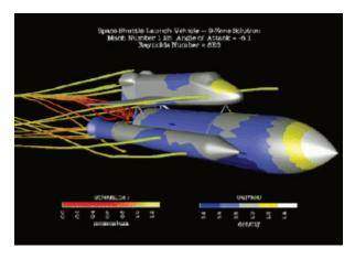
Momentum is shown as streamlines colored by magnitude and the density on the shuttle surface is shown as shaded contours – NASA Ames
