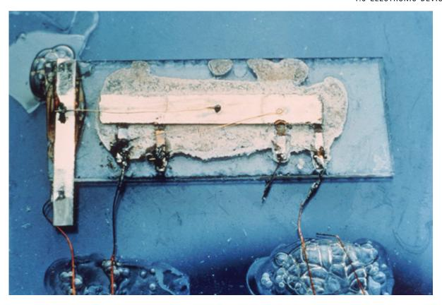
Kilby "monolithic" integrated circuit (source: Texas Instruments)
