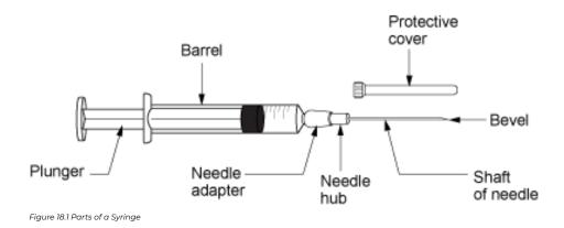
Luer lock syringes have threads in the needle hub that provide a secure connection of needles, tubing, or other devices. See Figure 18.2<sup>2</sup> for an image of a Luer lock syringe with a barrel and a readable scale. This image
