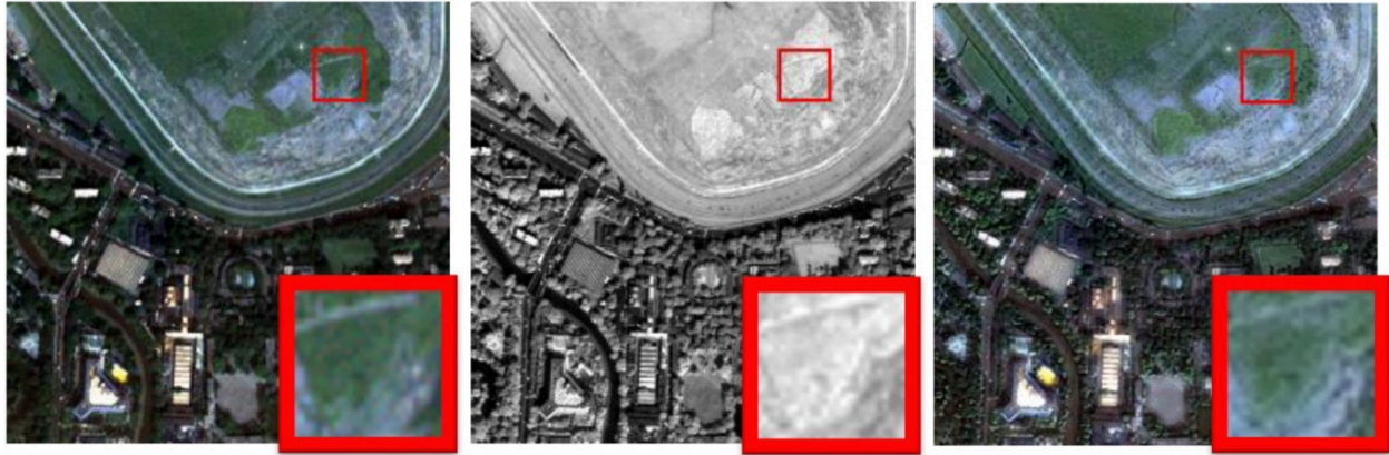
Figure 38: Illustration of pan-sharpening with a QuickBird Image. The true-colour image (left, 2.4 m resolution) is combined with the pan-chromatic image (center, 60 cm resolution) to produce the pan-sharpened image (right). Two-Path Network with Feedback Connections for Pan-Sharpener in Remote Sensing (Figure 7) by Fu et al, CC BY 4.0.
