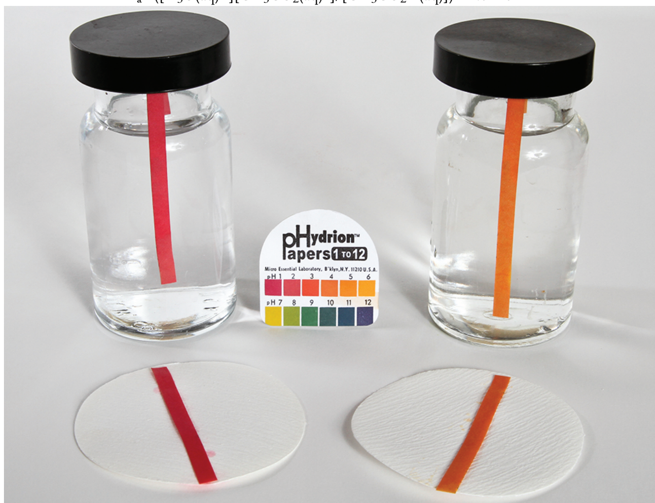
Figure 5.3.4. pH paper indicates that a 0.1 M solution of HCl (beaker on left) has a pH of 1. The acid is fully ionized and [\text{H}_3\text{O}^+] = 0.1 \text{ M} . A 0.1 M solution of \text{CH}_3\text{CO}_2\text{H} (beaker on right) is a pH of 3 ( [\text{H}_3\text{O}^+] = 0.001 \text{ M} ) because the weak acid \text{CH}_3\text{CO}_2\text{H} is only partially ionized. In this solution, [\text{H}_3\text{O}^+] < [\text{CH}_3\text{CO}_2\text{H}] . (credit: modification of work by Sahar Atwa)
