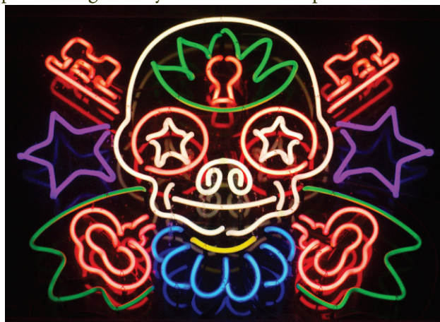
Figure 8.2.1. Neon signs operate by exciting a gas at low partial pressure using an electrical current. This sign shows the elaborate artistic effects that can be achieved. (credit: Dave Shaver)
