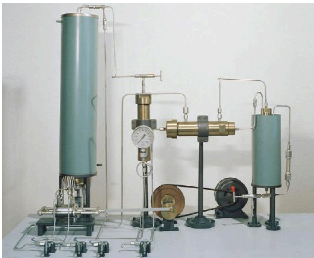
Figure 4.3.2. The original laboratory apparatus designed by Fritz Haber and Robert Le Rossignol in 1908 for synthesizing ammonia from its elements. A metal catalyst bed, where ammonia was produced, is in the large cylinder at the left. The Haber-Bosch process used for the industrial production of ammonia uses essentially the same process and components but on a much larger scale. Unfortunately, Haber's process enabled Germany to prolong World War I when German supplies of nitrogen compounds, which were used for explosives, had been exhausted in 1914.
