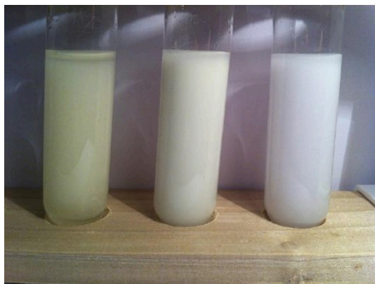
Figure 1.4.8. The three common silver halide precipitates: \text{AgI} , \text{AgBr} and \text{AgCl} (left to right). The silver halides precipitate out of solution, but often form suspensions before settling. Image used with permission (CC BY-SA 3.0; Cychr).
