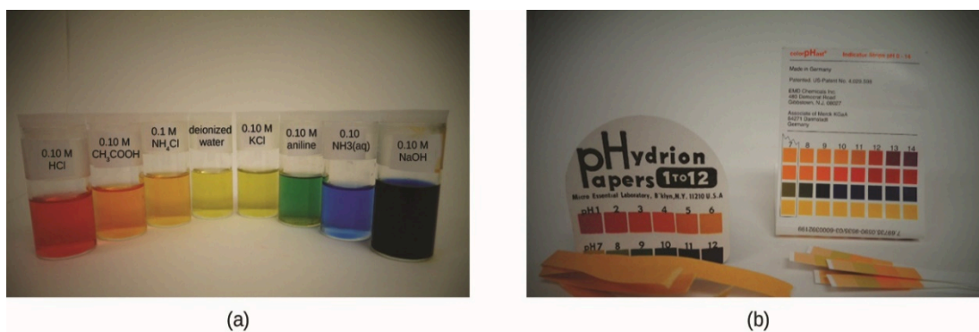
Figure 5.2.5. (a) A universal indicator assumes a different colour in solutions of different pH values. Thus, it can be added to a solution to determine the pH of the solution. The eight vials each contain a universal indicator and 0.1 M solutions of progressively weaker acids: HCl (pH = 1), CH 3 CO 2 H (pH = 3), and NH 4 Cl (pH = 5), deionized water, a neutral substance (pH = 7); and 0.1 M solutions of the progressively stronger bases: KCl (pH = 7), aniline, C 6 H 5 NH 2 (pH = 9), NH 3 (pH = 11), and NaOH (pH = 13). (b) pH paper contains a mixture of indicators that give different colours in solutions of differing pH values. (credit: modification of work by Sahar Atwa)
