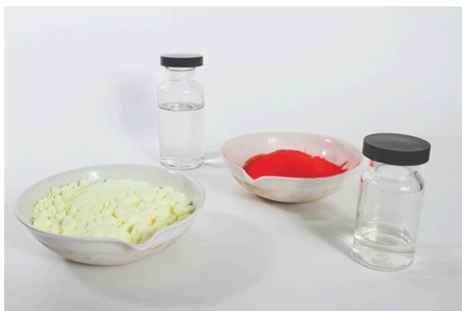
Figure 1.1.2. Each sample contains 6.02 \times 10^{23} molecules or formula units—1.00 mol of the compound or element. Clock-wise from the upper left: 130.2 g of \text{C}_8\text{H}_{17}\text{OH} (1-octanol, formula mass 130.2 amu), 454.4 g of \text{HgI}_2 (mercury(II) iodide, formula mass 454.4 amu), 32.0 g of \text{CH}_3\text{OH} (methanol, formula mass 32.0 amu) and 256.5 g of \text{S}_8 (sulfur, formula mass 256.5 amu). (credit: Sahar Atwa)
