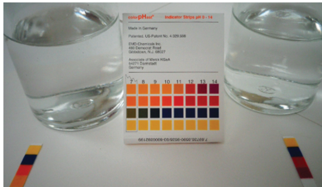
Figure 5.3.5. pH paper indicates that a 0.1 M solution of \text{NH}_3 (left) is weakly basic. The solution has a pOH of 3 ( [\text{OH}^-] = 0.001 \text{ M} ) because the weak base \text{NH}_3 only partially reacts with water. A 0.1 M solution of \text{NaOH} (right) has a pOH of 1 because \text{NaOH} is a strong base. (credit: modification of work by Sahar Atwa)
