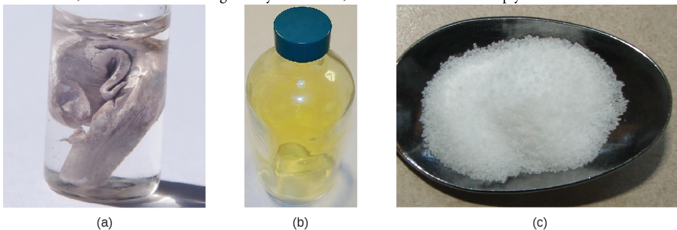
Figure 9.2.1. (a) Sodium is a soft metal that must be stored in mineral oil to prevent reaction with air or water. (b) Chlorine is a pale yellow-green gas. (c) When combined, they form white crystals of sodium chloride (table salt). (credit a: modification of work by “Jurii”/Wikimedia Commons)
