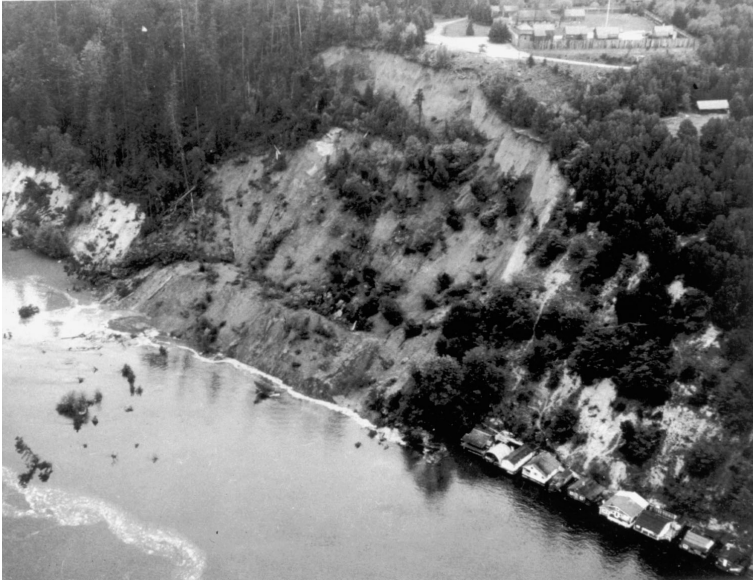
Figure 8-12a. Landslide on steep bluffs overlooking Puget Sound at Salmon Beach, near Tacoma Narrows, a few days after the 1949 Puget Sound Earthquake. The landslide endangered several beach houses and produced high waves in the narrows. Landslides occurred at the same place during the 2001 Nisqually Earthquake. From Washington Division of Geology and Earth Resources.
