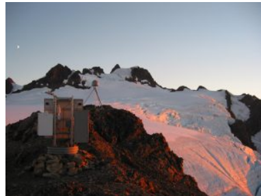
Figure 3-19. Global Positioning System (GPS) survey, part of the Pacific Northwest Geodetic Array (PANGA), of a rock outcrop on the Snow Dome on the north side of Mount Olympus, Olympic National Park. Photo by Spencer Reeder, Central Washington University
