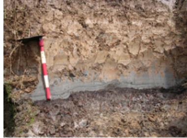
Figure 9-5a. Exposure at low tide of sediments below the modern tidal marsh at Willapa Bay, southwest Washington. The shovel blade is at the top of the dark soil layer marking a former marsh that subsided abruptly in A.D. 1700 during the last Cascadia Subduction Zone earthquake. The strongly layered sediments just above the soil layer are sands deposited by a tsunami that immediately followed the subsidence. Photo by Brian Atwater, USGS
