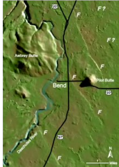
Figure 6-30. Computer-generated topographic map of Bend, Oregon, region showing young faults (linear features marked F). Image is illuminated by a light source from northeast that is 15 degrees above the horizon; accordingly, fault scarps that face northeast are brightly lit, whereas fault scarps facing southwest (such as the lineation marked F? north of Pilot Butte) are in shadow. These faults cut volcanic materials and sediments as young as late Pleistocene, but are not known to cut Holocene deposits. The prominence of these faults may be due to the greater consolidation of the deposits cut by them rather than their Holocene age. The fault scarp in
