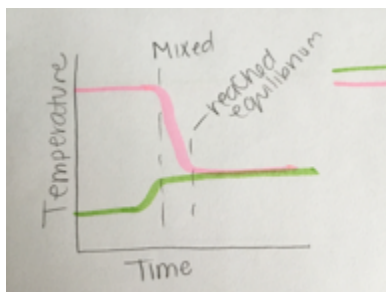
FIG. 2.16 Graph representing the mixing of hot and cold water. More hot water or more cold water?
