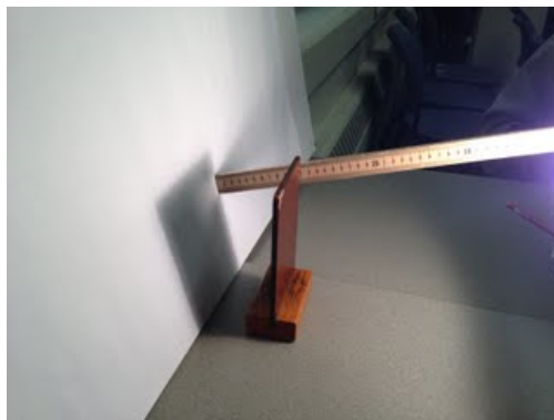
FIG. 1.7 A straight stick can provide a physical model for how light travels.
