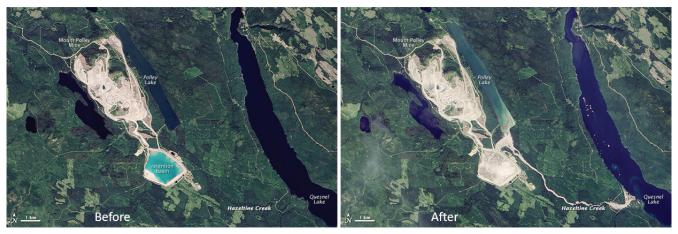
Figure 20.1.11 The Mt. Polley Mine area before and after to the dam breach of August 2014. The tailings were stored in the area labelled "retention basin." The retention dam failed and water and tailings released flowed into Polley Lake, Hazeltine Creek, and Quesnel Lakes.
