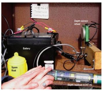
Figure 14.3.5 B.C. observation well 228 near Cassidy, Vancouver Island. The installation also has a solar panel, which is not visible in this view. [Image Description]
