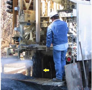
Figure 14.3.1 A water-well drilling rig in operation near Nanaimo, B.C. In the photo on the right the well is being test-pumped with air pressure. The casing (yellow arrow) is about 40 centimetres in diameter.
