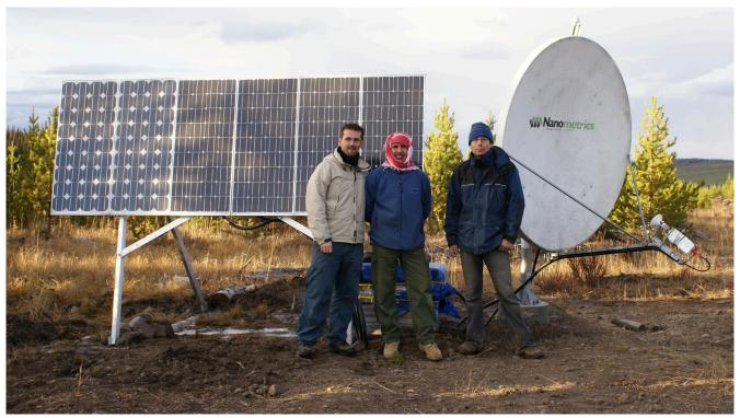
Figure 4.5.1 A seismometer and related power and communication equipment installed in 2007 in the vicinity of the Nazco Cone, British Columbia
