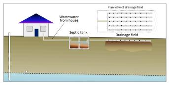
Figure 14.4.10 A typical septic system.
