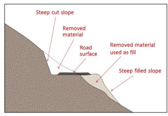
Figure 15.3.1 An example of a road constructed by cutting into a steep slope. The cut material was moved to outside part of the road to act as fill.
