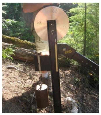
Figure 15.3.3 Part of a motion-monitoring device at the Checkerboard Slide near Revelstoke, B.C. The lower end of the cable is attached to a block of rock that is unstable. Any incremental motion of that block will move the cable, which will be detectable on this device.
