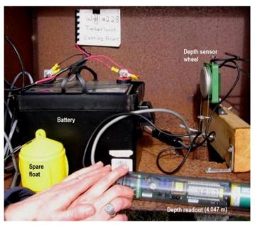
Figure 14.3.5 B.C. observation well 228 near Cassidy, Vancouver Island. The installation also has a solar panel, which is not visible in this view. [Image Description]
