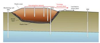
Figure 14.4.4 A cross-section of a typical modern landfill.
