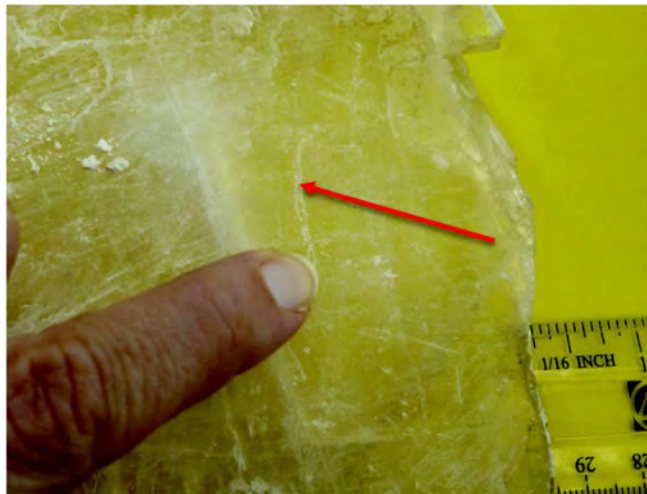
Figure 7.7 | An example of a scratch made by a fingernail on the mineral gypsum. The red arrow is pointing to the scratch. Gypsum, therefore, is softer than a fingernail.
