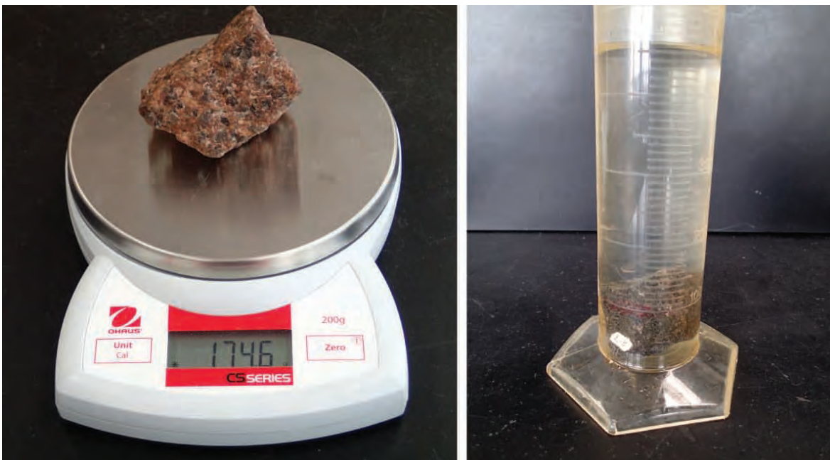
Figure 4.4 | Method to find the density of a rock. First the weight is measured on a digital scale and then the fluid displacement method is used to determine the volume.
