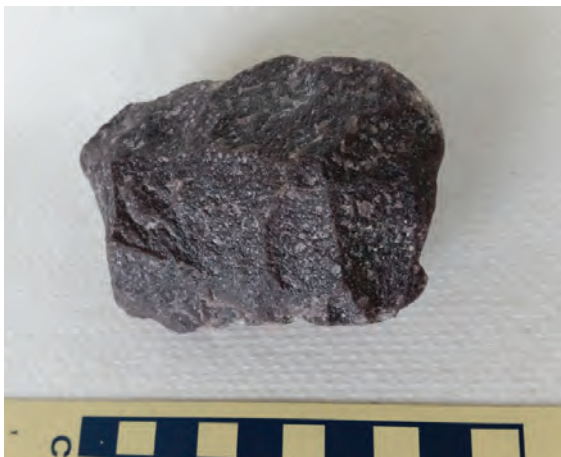
Figure 11.7 | An example of quartzite; a non-foliated metamorphic rock. Quartzite can appear in a variety of colors, but most are fairly light in color.
