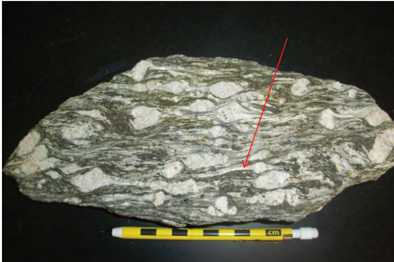
Figure 11.12 | Example of a mylonite rock; note the deformed light-colored minerals (feldspars) that have developed a tail (red arrow). The direction of shearing can sometimes be determined by examining these minerals.
