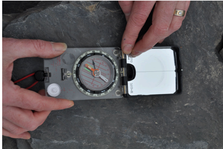
Figure 1: Compass used to measure an azimuth – in this case the strike of a bedding plane.
