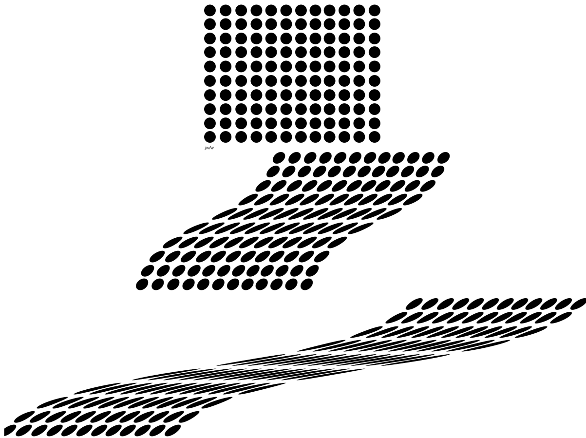
Figure 3. Simulation of heterogeneous simple shear applied to a grid of markers. Fabric produced as strain becomes more intense as it curves toward the centre of the shear zone.
