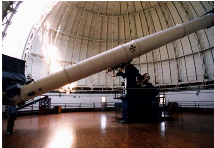
Figure 2.43 In 1897, the Yerkes Observatory in Wisconsin (USA) built a large refracting telescope with an objective lens that is 40 inches in diameter and has a tube length of 62 feet. (credit: Yerkes Observatory, University of Chicago)
