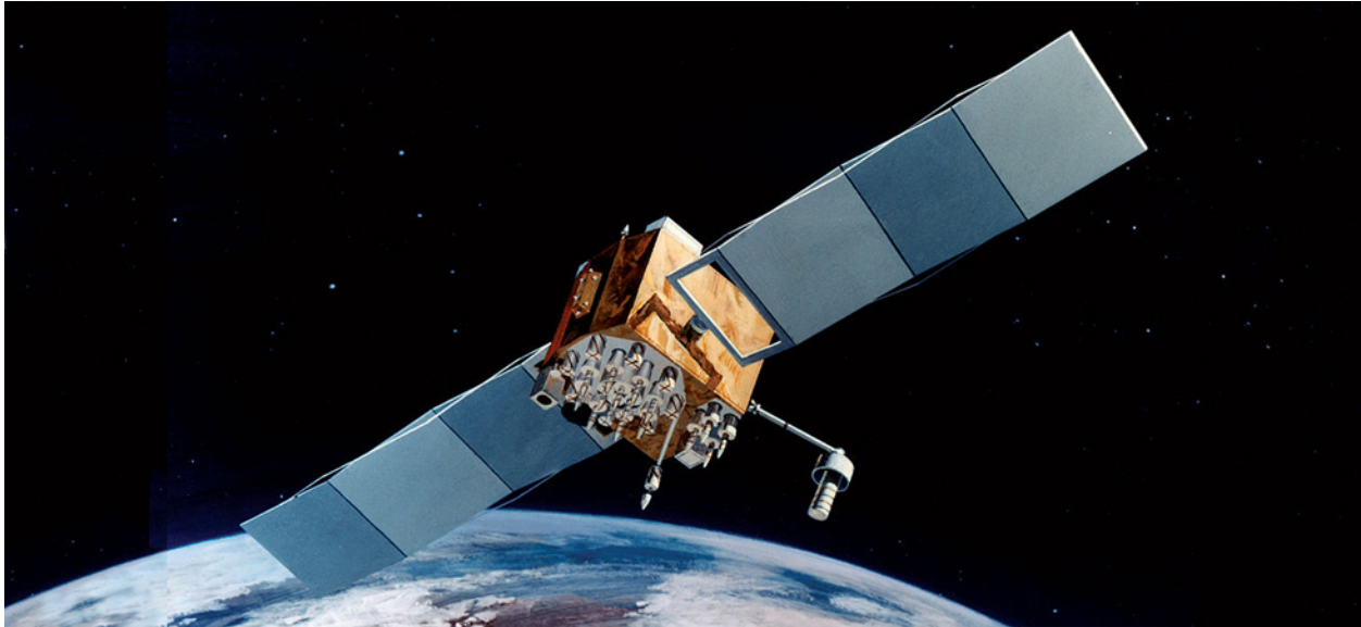
Figure 5.1 Special relativity explains how time passes slightly differently on Earth and within the rapidly moving global positioning satellite (GPS). GPS units in vehicles could not find their correct location on Earth without taking this correction into account. (credit: USAF)
