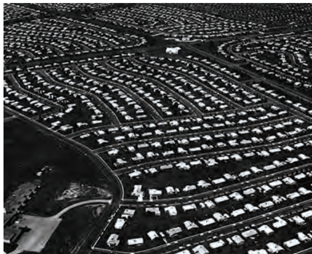
Figure 28.12 This aerial view of Levittown, Pennsylvania, reveals acres of standardized homes. The roads were curved to prevent cars from speeding through the residential community that was home to many young families.
