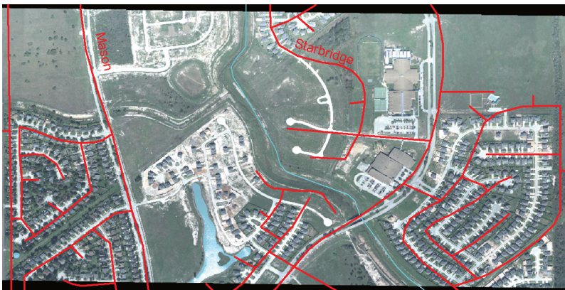
Discrepancy between pre-modernization TIGER/Line file streets (red) and actual geometry of street network shown in an orthorectified aerial image (U.S. Census Bureau n.d).
