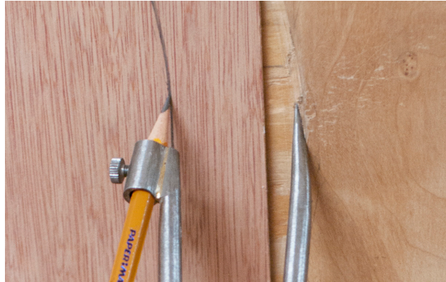
Figure 38 — Scribing an irregular line
