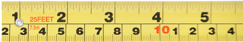
Figure 3—Tape measure with imperial on the top and metric on the bottom marked in 10 mm units
