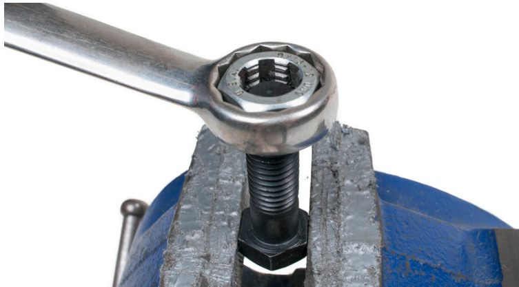
Figure 10 — Using a die nut
