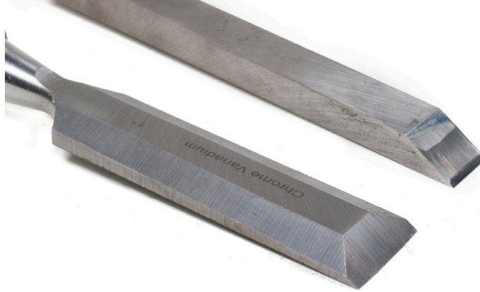
Figure 22 — Bevelled and straight-edge wood chisels
