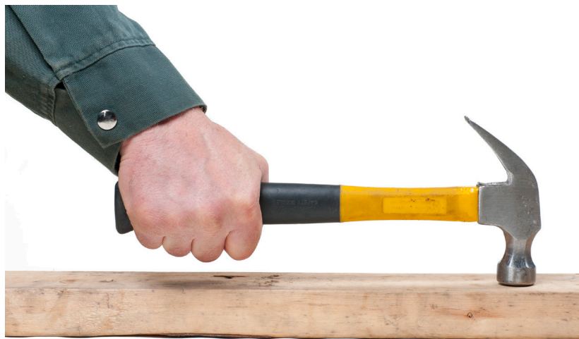
Figure 2 — When using a hammer, your knuckles must have clearance
