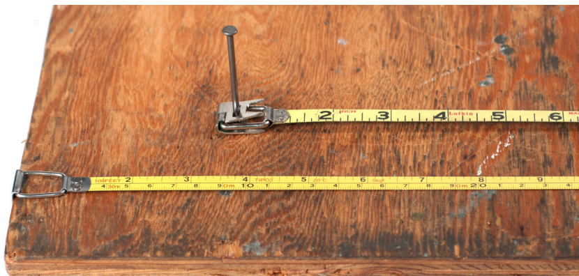
Figure 6—Hooks and rings at end of steel tapes
