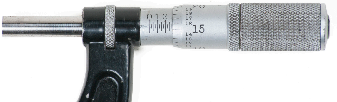
Figure 12 — Imperial micrometer reading 0.291 in.
