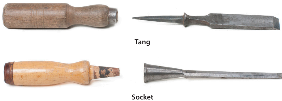
Figure 23 — Tang (top) and socket (bottom) chisels
