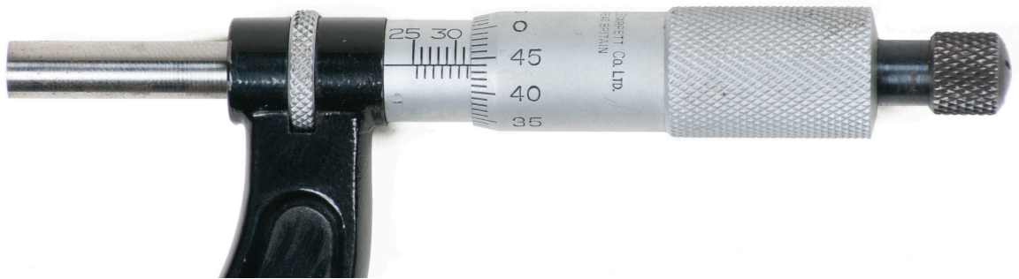
Figure 13 — Metric micrometer reading 31.94 mm
