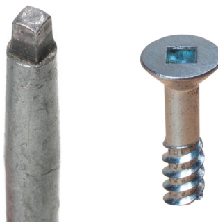
Figure 10—Robertson screwdriver tip and screw
