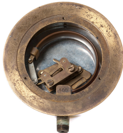
Figure 12 — Mechanical side of a pressure gauge showing the Bourdon tube
