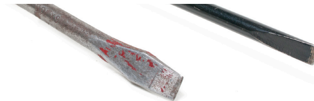
Figure 2 — Regular swaged-ended screw-driver (left); Cabinet-tip straight-ended screwdriver (right)
