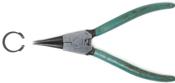
Figure 23 — Snap-ring pliers with internal circlip
