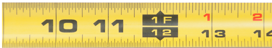
Figure 2 — An imperial tape with divisions of \frac{1}{2} and \frac{1}{16} of an inch
