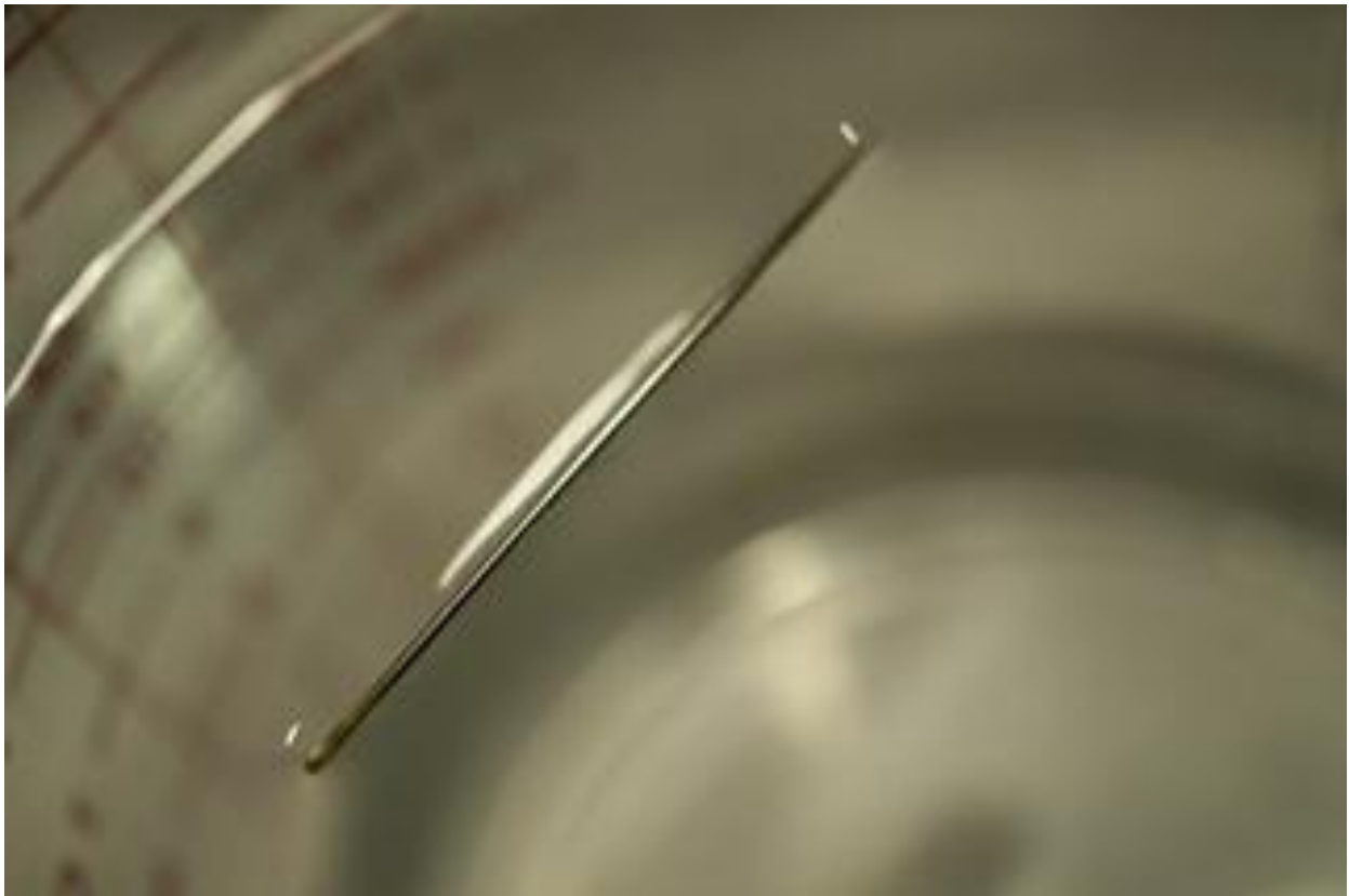
Figure 2.13 The weight of the needle is pulling the surface downward; at the same time, the surface tension is pulling it up, suspending it on the surface of the water and keeping it from sinking. Notice the indentation in the water around the needle. (credit: Cory Zanker)
