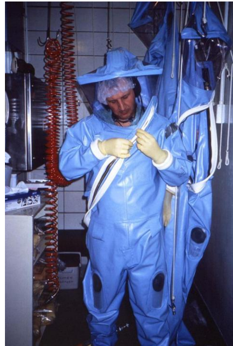
Figure 6.10 Positive pressure suit used in biosafety level 4 laboratories and other level 4 settings.
