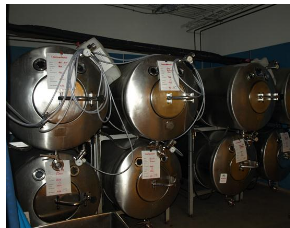
Figure 8.37 Alcohol Fermentation Fermentation of grape juice into wine produces CO 2 as a by-product. Fermentation tanks have valves so that the pressure inside the tanks created by the carbon dioxide produced can be released.
