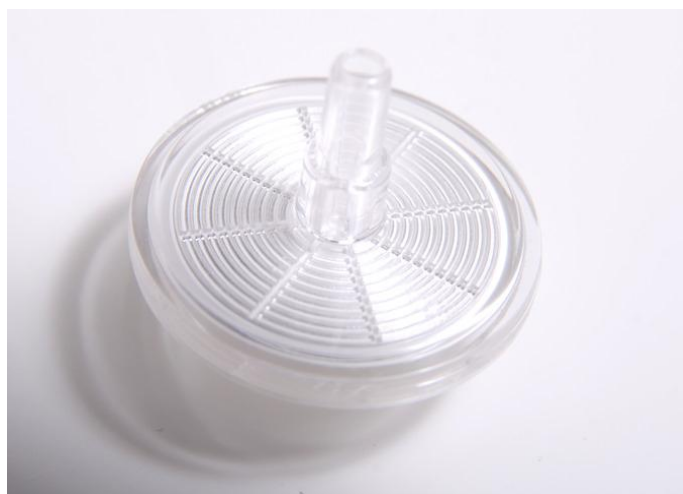
Figure 6.40 Syringe Filter A syringe filter with a pore size of 0.22 micrometers, small enough to capture and retain bacterial and fungal cells.
