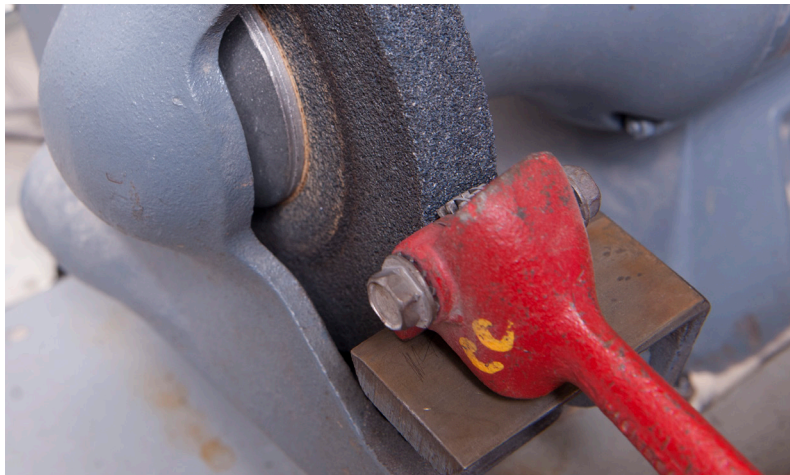
Figure 12 — Using a wheel dresser
