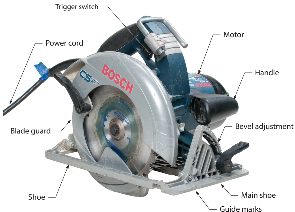
Figure 1 — Portable circular saw
