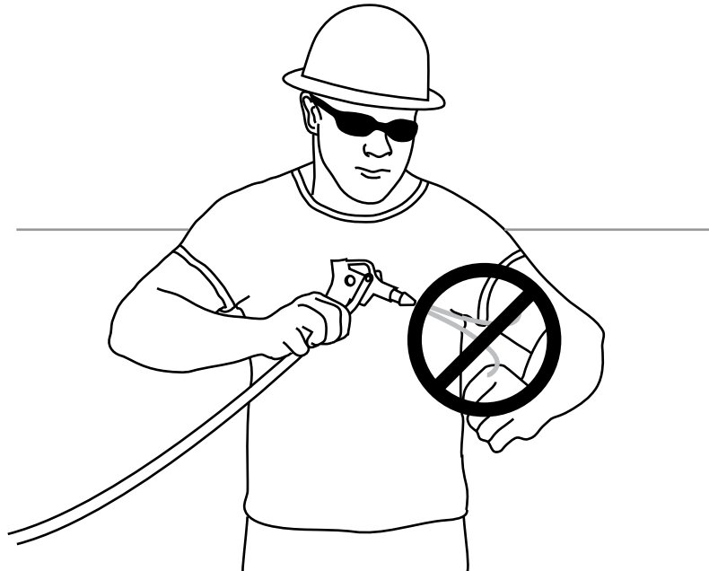
Figure 8 — Do not clean yourself with compressed air
