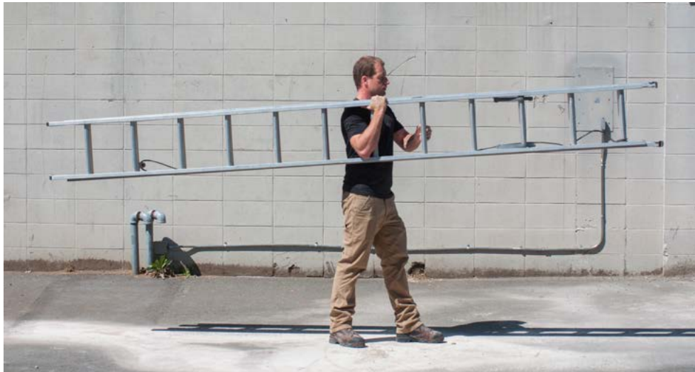
Figure 2 — Lifting a ladder
