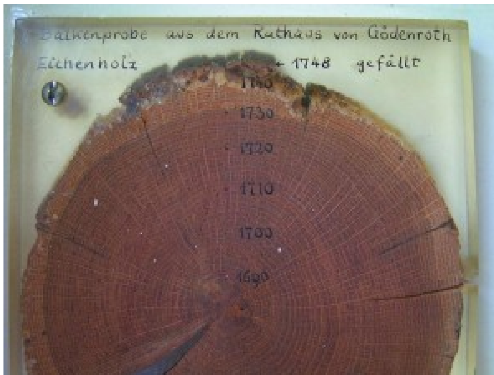
Dendrochronology: tree ring dating. “Dendrochronologie” by Stefan Kühn is licensed under CC BY-SA 3.0.
