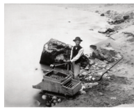
Figure 13.31 Chinese miners introduced machinery like this “rocker” on the Fraser River ca. 1875.
