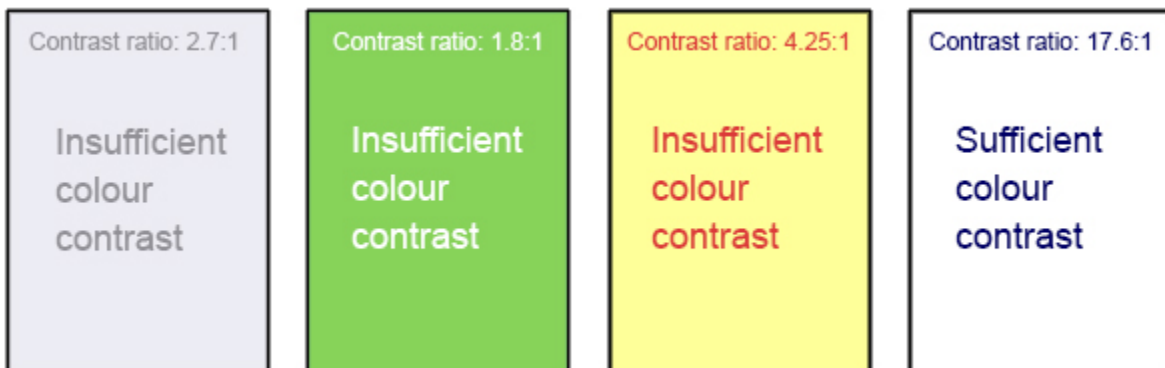
The image displays four examples of foreground (text) colour against background colours; only the example on the far right presents combinations with sufficient colour contrast.
