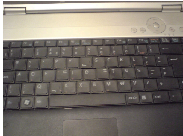
Figure 11.5.4: Dvorak keyboard is a more efficient alternative to keyboard design. However, due to resistance from typists, teachers, manufacturers, and salespeople, a switch never occurred. “Sony laptop with Dvorak keyboard layout” by John Blackbourne, licensed under CC BY-NC 2.0.
